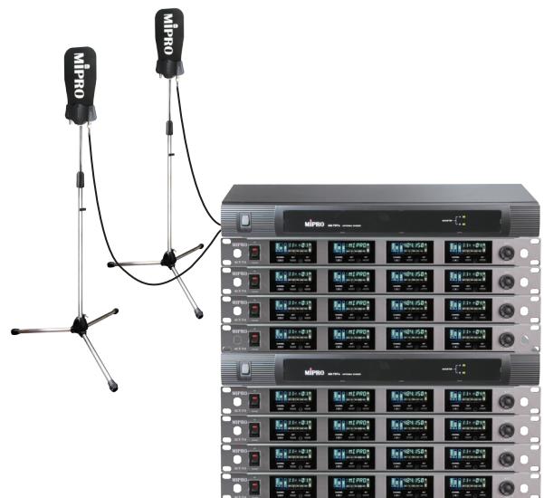
Figure 11: Two AD-707a wideband antenna dividers with eight quad-channel receivers to form a 32-channel system.
