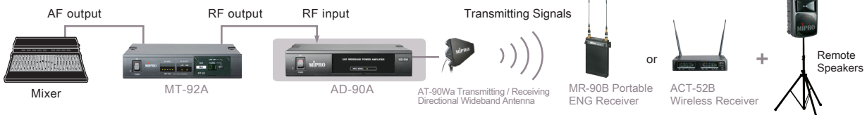
Application of AD-90S with MI-808T Stereo Transmitter & AT-90Wa Transmitting / Receiving Directional Wideband Antenna
