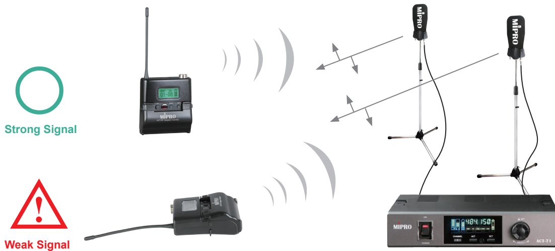
Figure 2: How the signal quality is presented between the linearly polarized antennas.
