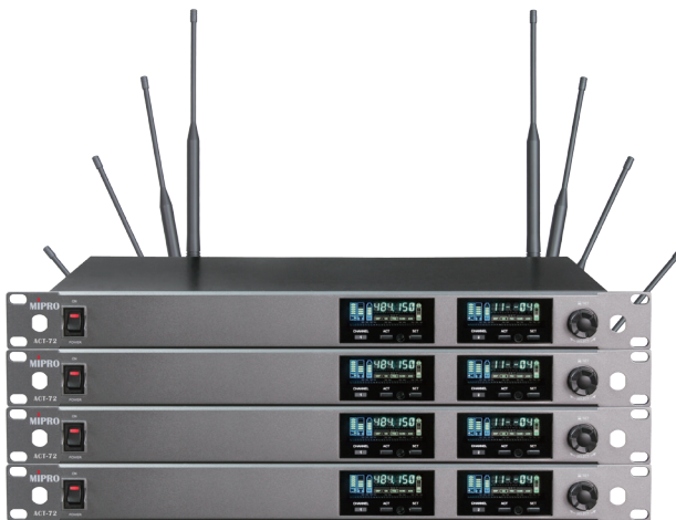
Figure 1A: Antenna installation with four dual-channel receivers.
