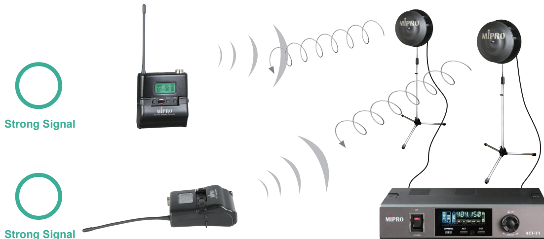
Figure 3: How the signal quality is presented between the linear and the circular polarization antennas.
