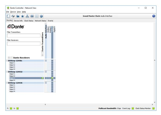
All Dante™ input interface parameters (e.g. the audio routing within a Dante network) must be configured with the Dante Controller software.
