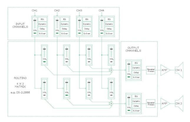
Fig. 2: Four input channels are mixed to two output channels.
