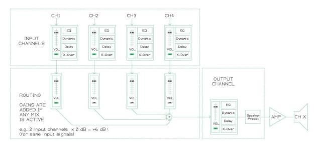
Fig. 1: Four input channels are mixed to one output channel.
