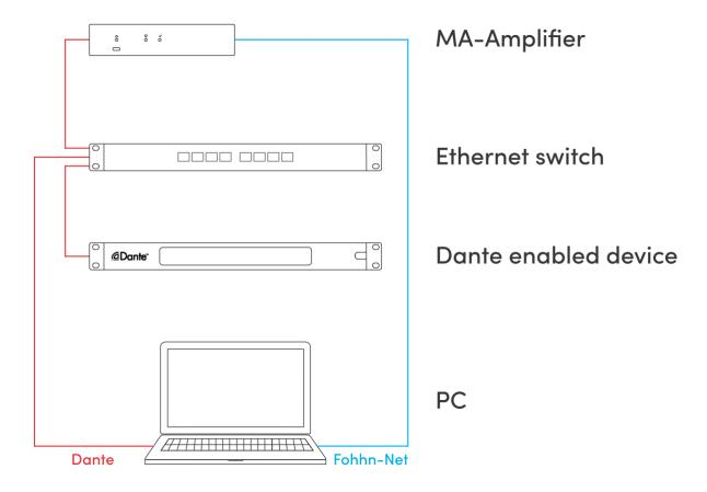
Example: Control of MA-Series amplifiers via computer and Ethernet switch using simple cabling.
