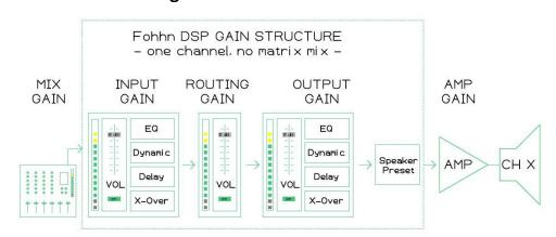
Fig. 1: Overview of the signal chain on a MA-Series amplifier channel
