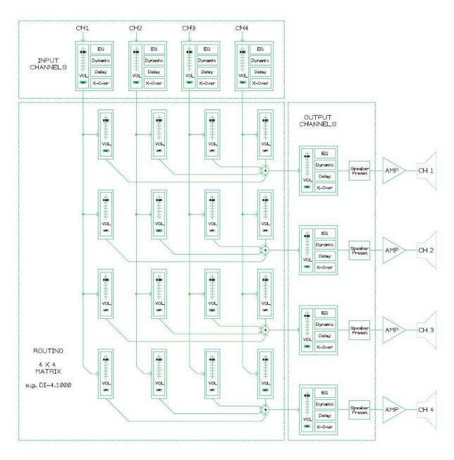
Fig. 3: Four input channels are mixed to four output channels.
