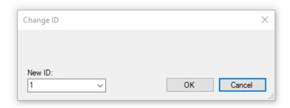
You can also change the ID of a **FOHHN** amplifier at any time while it is in use. To do this, the system must be in the **FOHHN-NET**. Proceed as follows:
